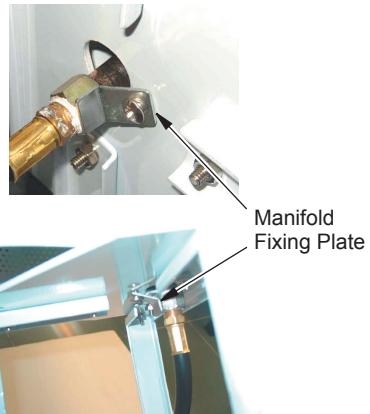
Figure 7 - Attaching Manifold Fixing Plate to Post Support
